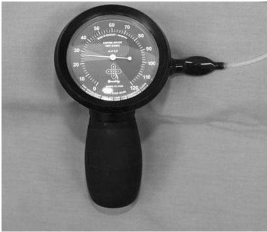
Fig. 5-46 Cuff Manometer. For low-pressure high-volume cuffs, a cuff manometer is used to inflate the endotracheal tube cuff and simultaneously measure the inflation pressure. Credit: Courtesy of Moses Goddard, M.D.
