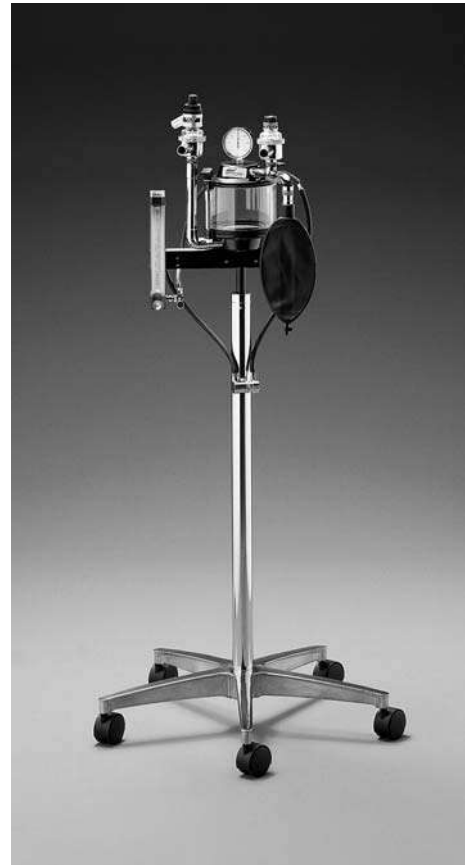
Fig. 5-24 Matrix VMS. This anesthesia machine is a pole-mounted compact machine. The APL valve is seen on the left mounted on the expiratory valve. The fitting on the right, atop the inspiratory valve, is a negative pressure relief valve or air intake valve, used to entrain room air if the oxygen supply fails. The breathing system manometer is placed on the absorber system. The vaporizer, not shown, is mounted below the absorber assembly. Credit: Courtesy of Matrix by Midmark.
