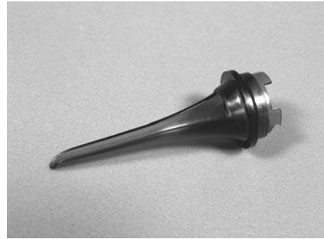
Fig. 5-44 Rat Intubation Speculum. The intubation speculum is similar to that described by Tran and Lawson (1986) and is molded of hard, autoclavable plastic for use with an operating head otoscope. Credit: Courtesy of Hallowell EMC.
