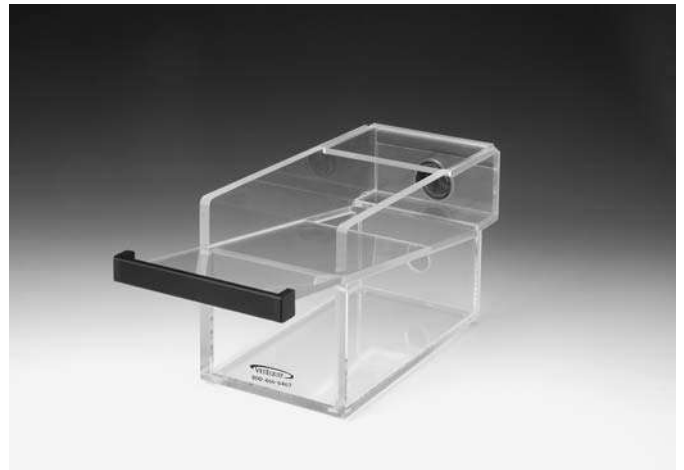
Fig. 5-34 VetEquip 2 l Vented Chamber. The sliding, inclined lid is seen at the left, opening into the chamber. A hood partially enclosing the evacuation connection is visible at the upper right. Anesthetic gases are introduced through a port located beneath the evacuation port in the wall of the chamber. As the lid is opened, the evacuation flow entrains gas from the chamber, conducting it away from the work area via a fan-driven high flow evacuation system. Credit: Courtesy of VetEquip, Inc.
