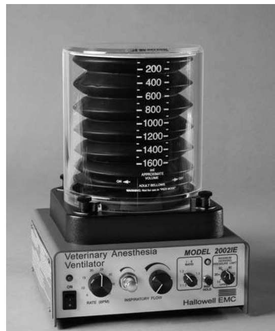
Fig. 5-28 Standing Bellows. The controls for this standing bellows anesthesia ventilator include, from left to right, the power switch, respiratory rate adjustment, fine and coarse inspiratory flow, adjustable I:E ratio, and the maximum working pressure control. Interchangeable bellows and housings can accommodate tidal volumes up to 3,000 ml. Credit: Hallowell EMC.
