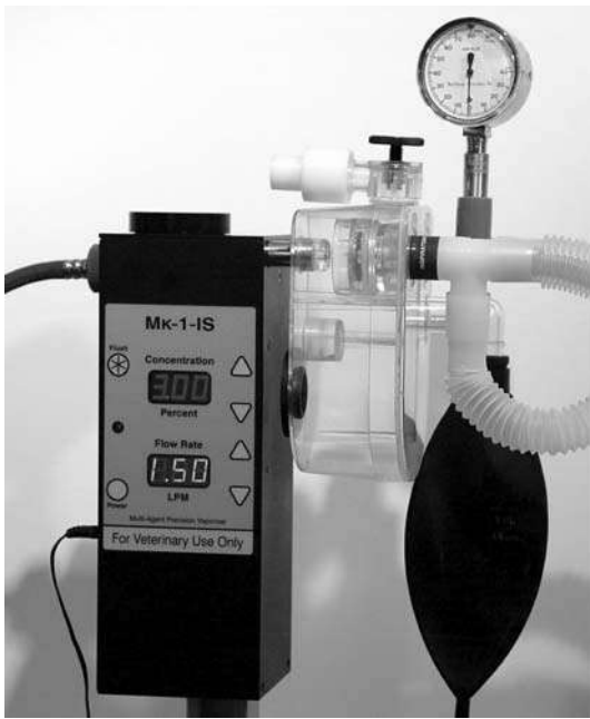
Fig. 5-11 MK-1-IS Veterinary Anesthesia Machine. The vaporizer and flowmeter module is seen at the left. Note the touch-sensitive control panel. In the center is a clear plastic absorber assembly with integrated unidirectional valves, APL valve with scavenging connection (top), and reservoir bag port. The breathing system manometer is seen at the top right, as well as the breathing circuit connections. Credit: Courtesy of Mark Kenny Products Company, LLC.
