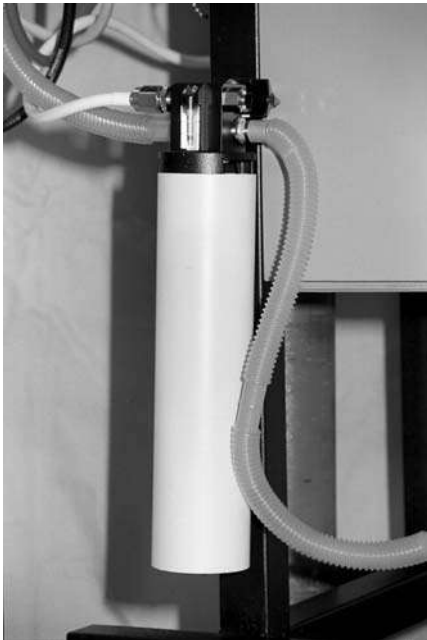
Fig. 5-13 Open Interface Scavenging System. This example is designed for a central vacuum system. The vacuum adjust needle and flowmeter are seen at the top. The white hose connects to the central vacuum scavenging system, and the two corrugated hoses are connected to the APL valve scavenging port, and the ventilator relief valve. The cylinder is a rigid reservoir. The openings to the room are not visible in this photograph.
