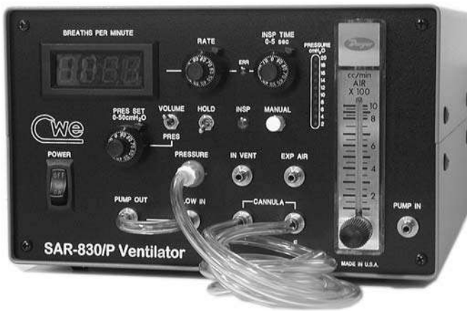
Fig. 5-32 CWE SAR-830/P Ventilator. From the top left, the display for ventilation rate, the rate control, the inspiratory time control, and a circuit pressure display are seen. The fresh gas flowmeter is at the far right. The second tier of controls and indicators include the power switch, adjustable maximum working pressure limit, a volume/pressure mode selector switch, an inspiratory hold control, and cycle mode indicators lights. The bottom tier includes pump and breathing circuit connections. Credit: Courtesy of CWE, Inc.
