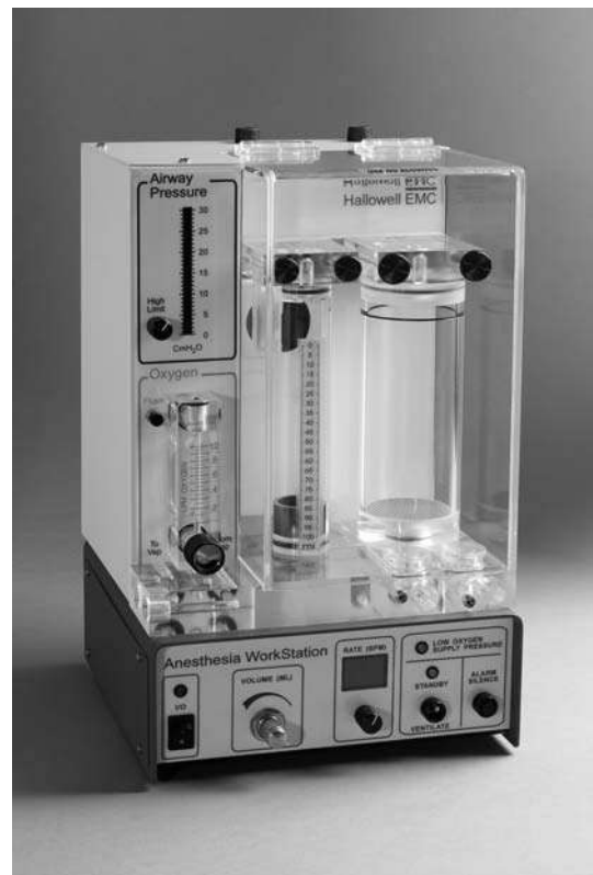
Fig. 5-30 Hallowell EMC Anesthesia Workstation. At the base of the ventilator from left to right, are the controls for power, tidal volume, and respiratory rate. The controls at the right include a standby switch and alarms. Airway pressure is indicated by an illuminated bar display at the top right, and the maximum working pressure is set using the adjacent dial. The oxygen flowmeter is seen below. The clear housing encloses the “bellows” seen to the left, and the absorbent canister and unidirectional valves, seen to the right. Credit: Courtesy of Hallowell EMC.
