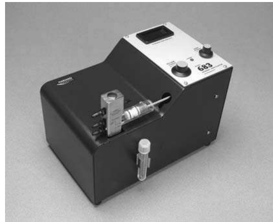
Fig. 5-31 Harvard 683 Small Animal Ventilator. This type of ventilator is commonly used for rodents and, in larger models, for many other research animals. Respiratory rate and tidal volume are set using the two dials seen to the right. Respiratory rate is indicated in the digital screen at the top right. The breathing circuit and fresh gas connections are housed in the valve tower seen at the lower right, with the waste gas connection on the opposite (top right) side of the valve tower. The piston assembly is to the lower left side of the valve tower. Credit: Courtesy of Harvard Apparatus.
