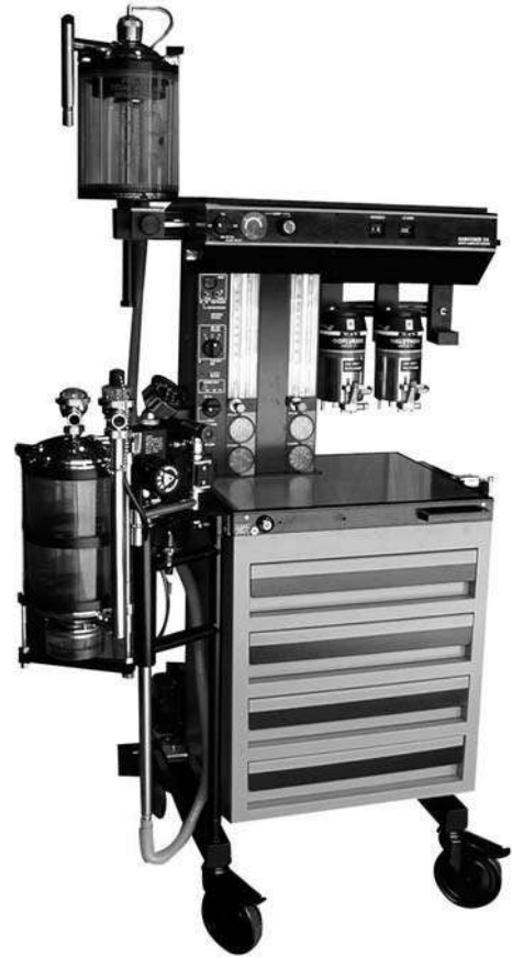
Fig. 5-26 North American Dräger 2A. The large work and storage space, multiple flowmeters, central supply and small tank pressure gauges, mounts for three vaporizers, and dual canister absorber system, are typical for machines of this series. Adjustable alarms for the breathing circuit are also common. Credit: Courtesy of DREVeterinary ( www.dreveterinary.com ).
