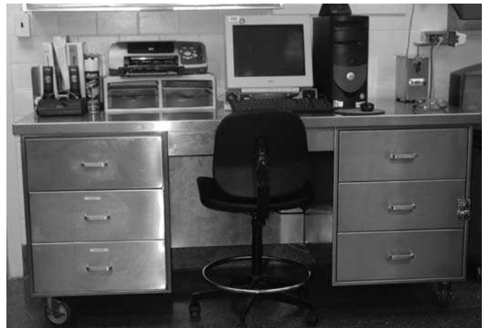
Fig. 9-3 An example of a stainless steel cabinetry used in the large-animal postprocedural care unit. The cabinet is manufactured with stainless steel casters for ease of maintaining sanitation. (Courtesy of the National Institutes of Health Veterinary Resources Program.)
